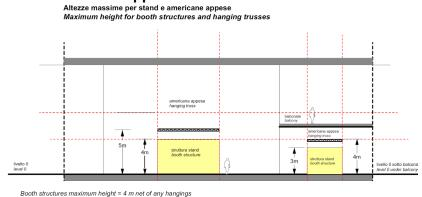
Booth structures maximum height = 4 m net of any hangings Booth structures under balcony maximum height = 3 m net of any hangings Maximum height of the trusses (excluding the area under the balcony) = 5 m upper side truss Maximum height of the trusses under balcony = 4 m upper side truss
